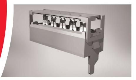
For the wire connection, a well-known AMP-LATCH type blade with a single slot is used. The insides of the slots are tin plated for stable and reliable connections.
