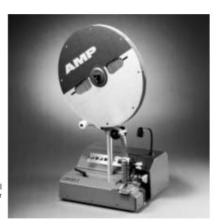
**Semi automatic tooling PN 677410-1.** This tool can be used for Micro-MaTch lead end and for daisy chain assembly applications.
