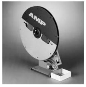
Connector dispensor PN 677463-1. The dispensor accepts the Micro-MaTch standard reels (2500 pcs/reel). It automatically removes the pre-set connector quantity from the reel and drops it in a separate box. Quantity can easily be programmed by the user.
